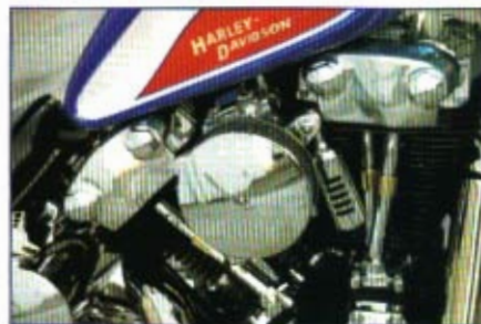
A Knucklehead or a Twin Cam? Well, both, sort of. The TC88 was stretched to 95 inches, then topped with Elvis's Place Knuckle rocker covers.
